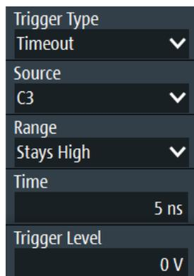
*Figure 2-18: Timeout trigger*
