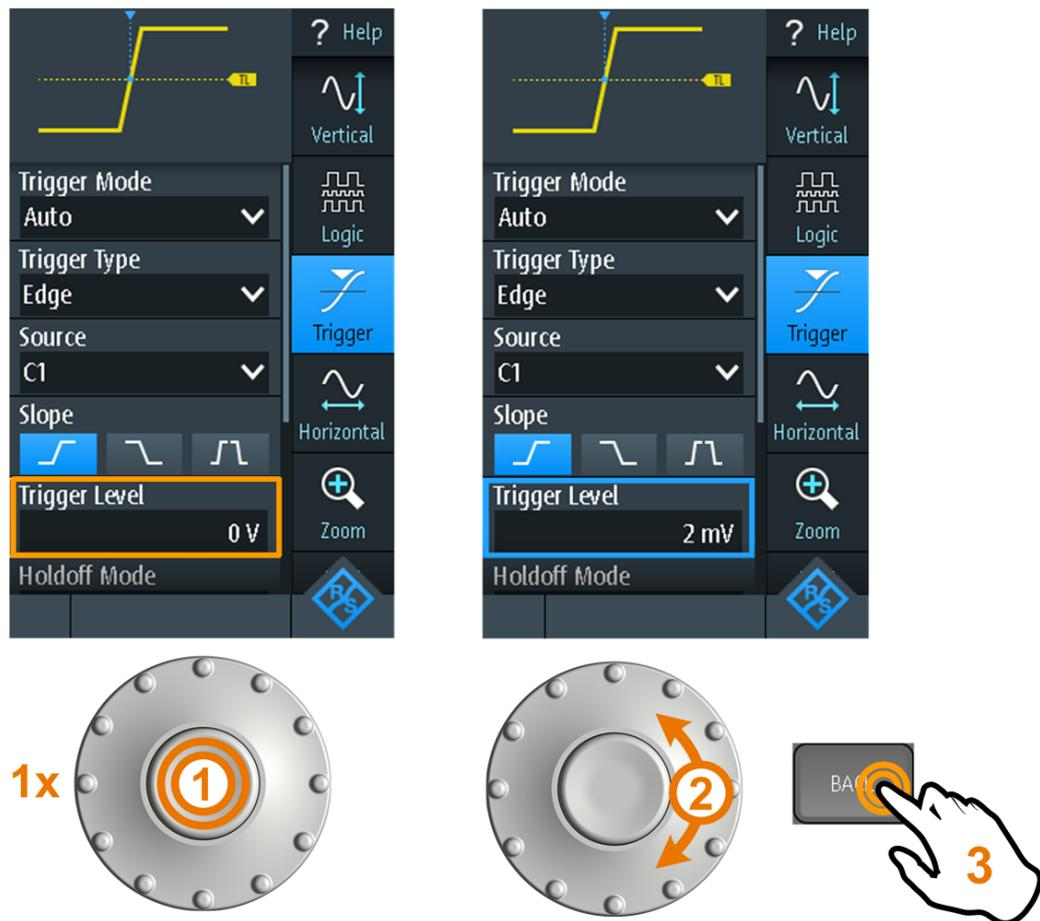
Figure 1-11: Set numerical value using the wheel
