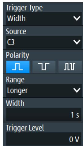
Figure 2-3: Width trigger
