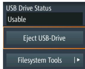
2. To remove the USB flash drive from the instrument, tap "Eject USB Drive" in the "File" menu.
