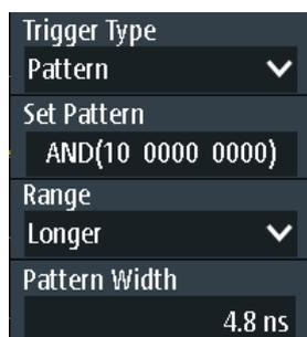
*Figure 2-10: Pattern trigger*
